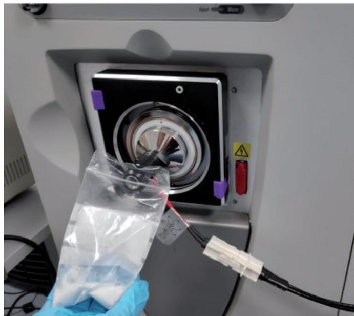
Figure 1 - Direct MS analysis of sample headspace via SICRIT<sup>®</sup> (shown on Thermo LTQ Orbitrap).
