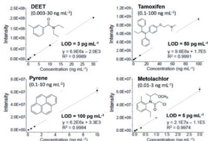
Figure 2 - Calibration curves for DEET, Tamoxifen, Pyrene, and Metolachlor in water, obtained with direct SPME-SICRIT<sup>®</sup>-MS.[2]
