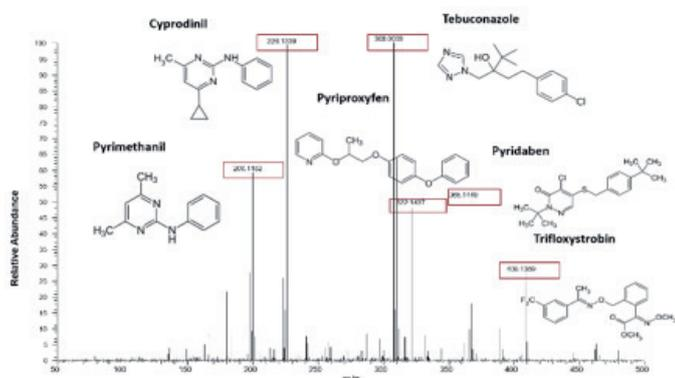
Figure 3 - HRMS full scan of a soil sample spiked with pesticides.
