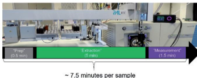
Figure 1 - Experimental setup and workflow of direct SPME-MS.
