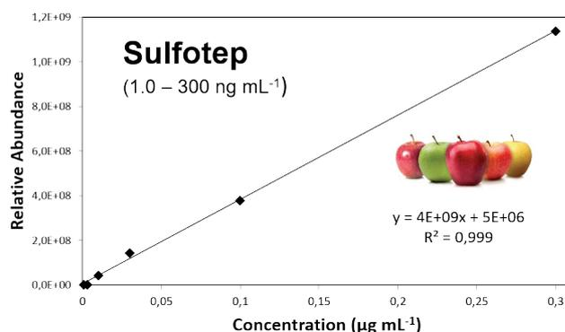
Figure 4 - Calibration curve of sulfotep in apple samples, obtained with direct SPME-SICRIT<sup>®</sup>-MS.
